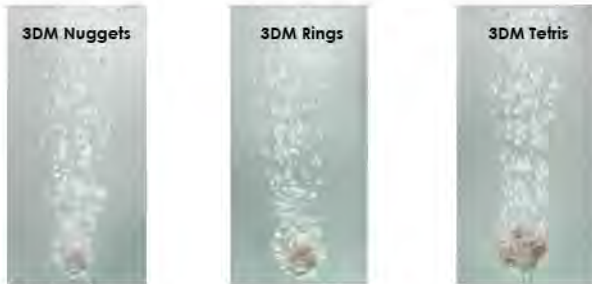
Experiment: Fine bubbles passing through fine cavities and micro-tunnels
