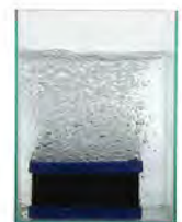
Rapid sizzling caused by microbubbles from micro-cavities
