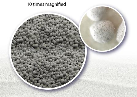
Cross section showing cavities.
